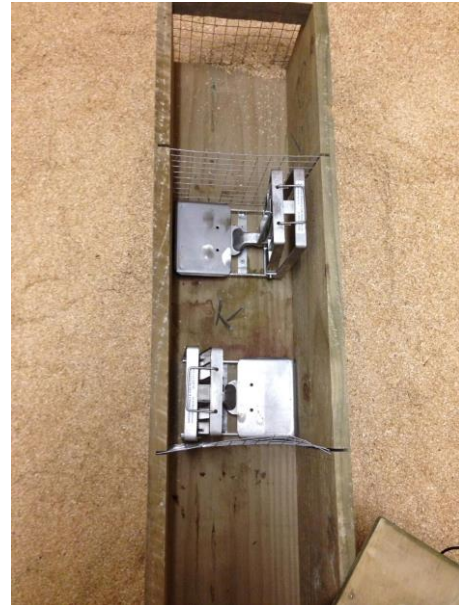
Figure 1.2: Internal view of BT200 trap tunnel showing double set BT200 traps and wire mesh baffles
