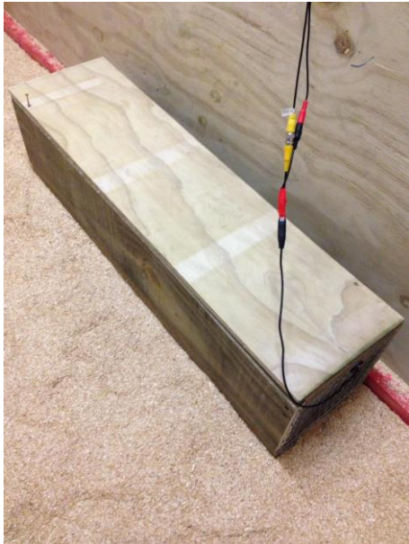
Figure 1.1: Outside view of BT200 trap tunnel
